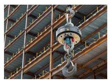
The IoT sensor that captures and analyzes thousands of data points on the flow and handling of site materials.
