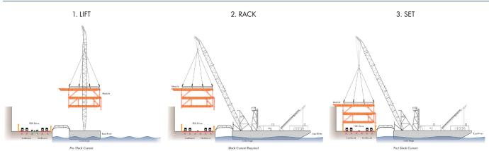
Diagram of each modules three basic movements
