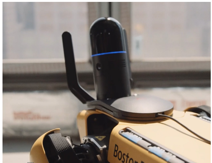
Spot can be outfitted with a variety of technological integrations including the Leica BLK ARC depicted above. The BLK ARC is a laser scanner made for autonomous robots like Spot.
